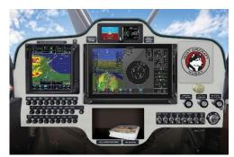
engine analytics and a GTN 750 Nav/Comm/GPS, this is the most capable, attractive and intuitive flight deck ever found in a Husky. There's even a **new glove box** and **device storage cubby**.
